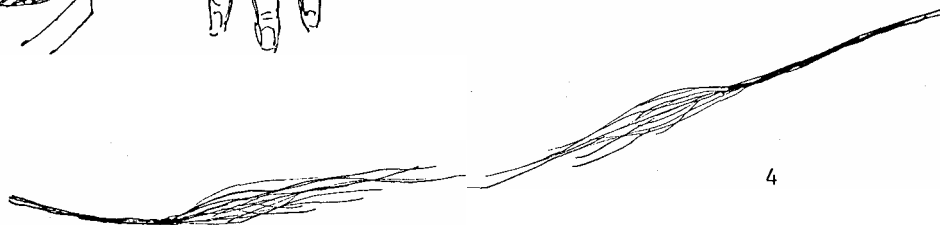
Fig.4. The thread does not come apart with a pop, or snap, or with any pressure at all. In the hand of a saddler it seems to float apart leaving the ends long, silky and tapered.
