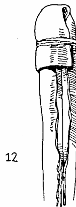
Fig. 12. If the tube is of canvas it is turned inside out as soon as it is made to hide the seam. If it is of leather this will usually be too difficult, so the seam should now be spread out and smoothed flat.
