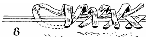
Fig. 8 When finishing go through the last hole twice at the front and bring the end up between the two pieces of leather.
